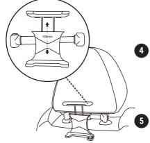
Insert the Switch Console into the Car Mount by extending the front Clamp. This mount is designed to fit devices up to 108mm high.
